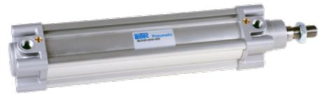
Double acting Al-profile cylinder with integrated sensor grooves, adjustable cushions and magnetic piston for proximity sensors. The sensors can be installed directly into the sensor grooves of the Al-profile. Standard stroke lengths in table below, additional lengths on request.
